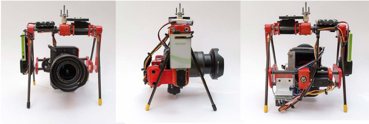
KAP Cradle No. 12: a three-axis, radio-controlled rig carrying an EOS-M3 camera with a 11-22mm lens.
